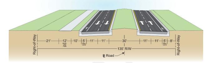
Figure 6-3: Nolte Road Extension Typical Section
