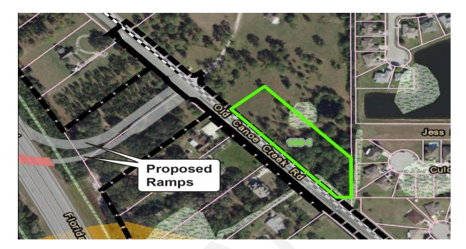
Figure 6-5: Proposed Pond Location at Old Canoe Creek Road Partial Interchange
