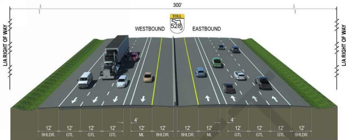
Figure A-2 Beachline Expressway Managed Lane Typical Section
