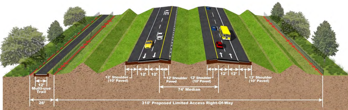
Figure 1-4 Roadway Typical Section
