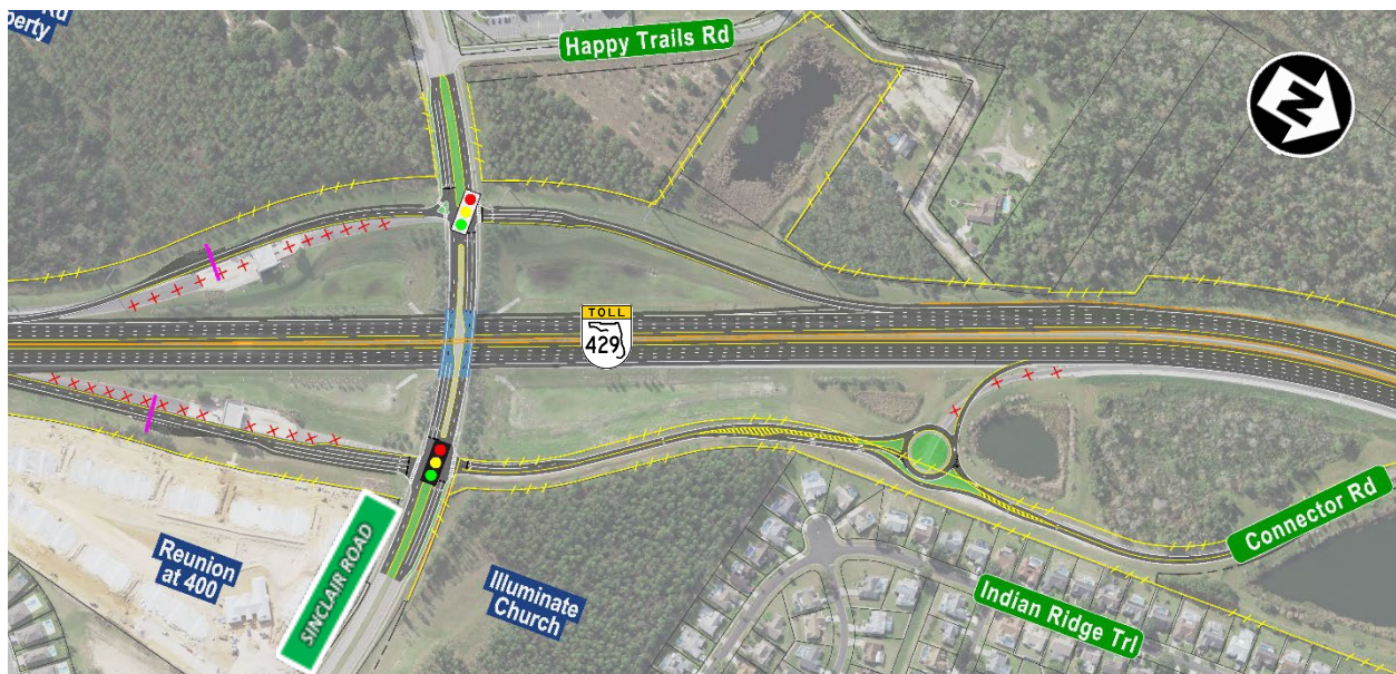
Figure 4-5: Sinclair Road Alternative 2 Roundabout
