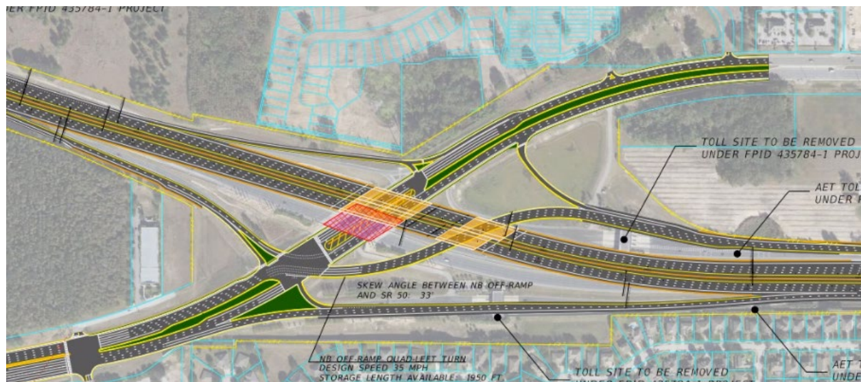
Figure 4-10: Example of Partial Parallel Flow Interchange
