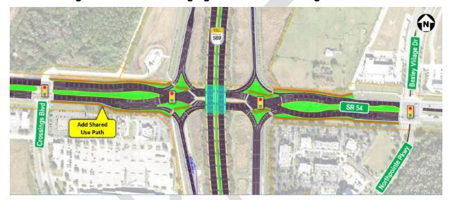
Figure 5-6: SR 54 Diverging Diamond Interchange Alternative
