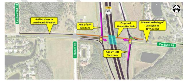
Figure 5-3: Van Dyke Road Interchange Alternative
