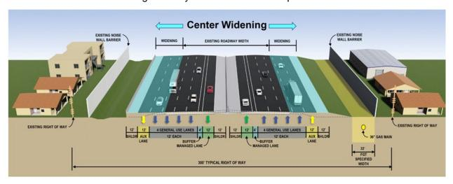
Figure 1-4 - Typical Section Segment 1
