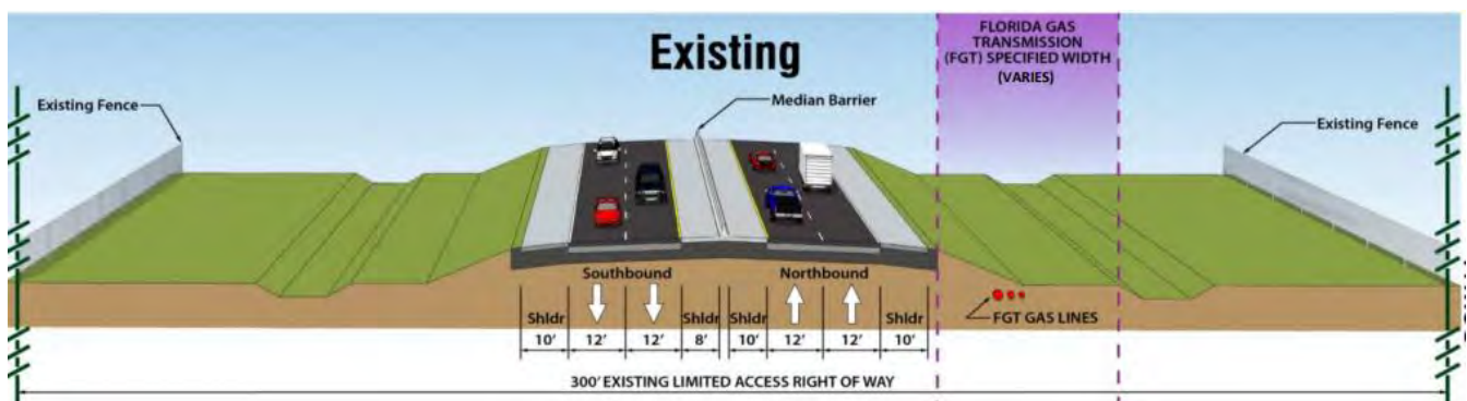
Figure 3: Existing Mainline Typical Section
