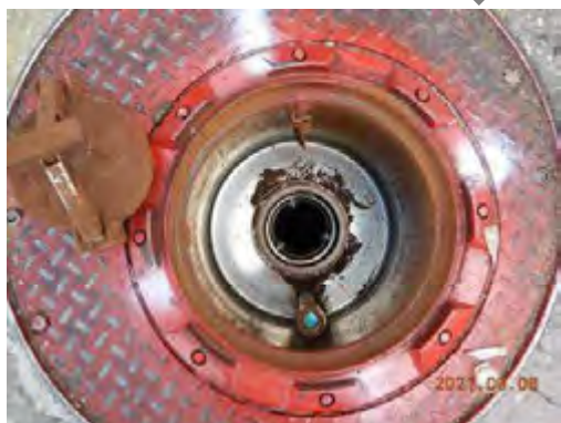
2021-09-08 New stainless steel insert in premium bucket
