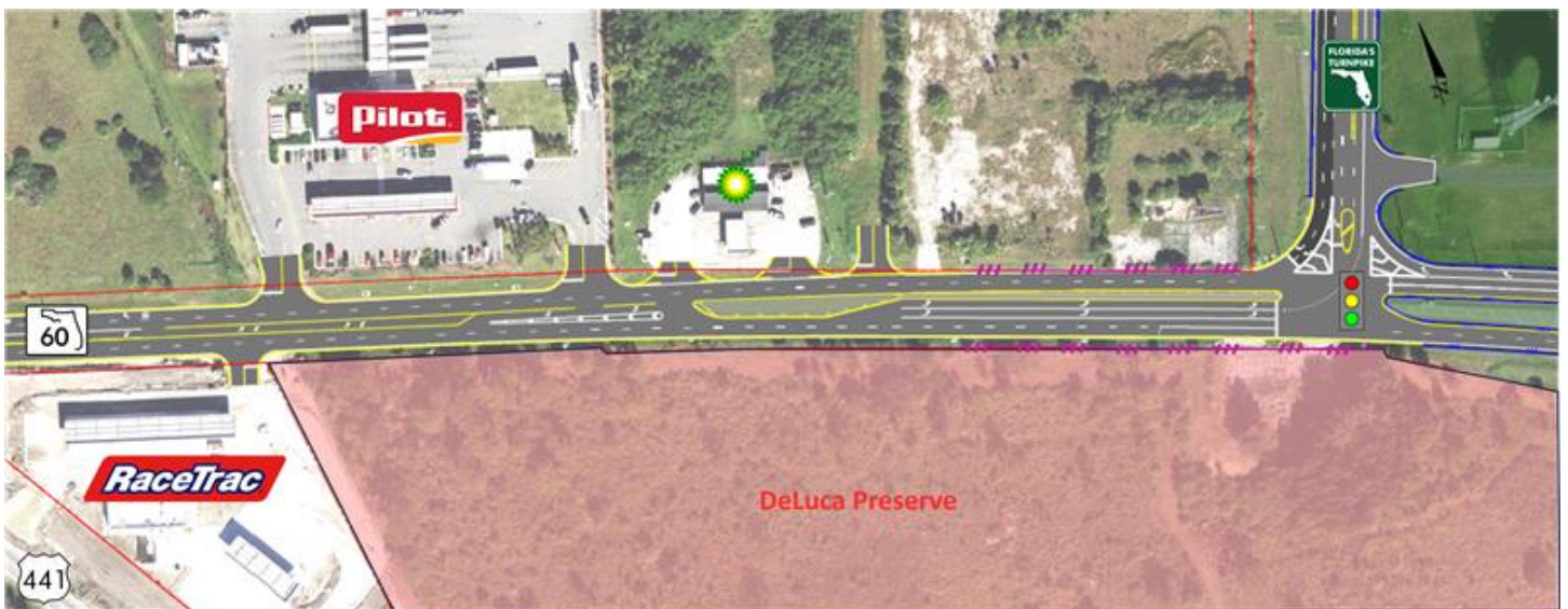
Figure 5: SR 60 Access Modifications
