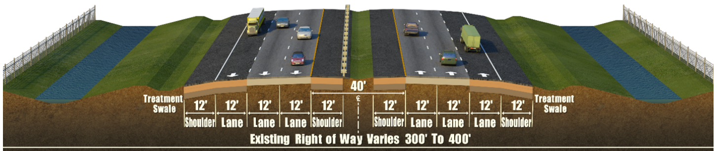
Figure 3: Preferred Typical Section Alternative (Looking North)
