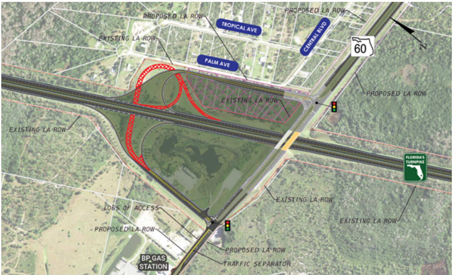
Figure 4: Improvements at the SR 60 Interchange
