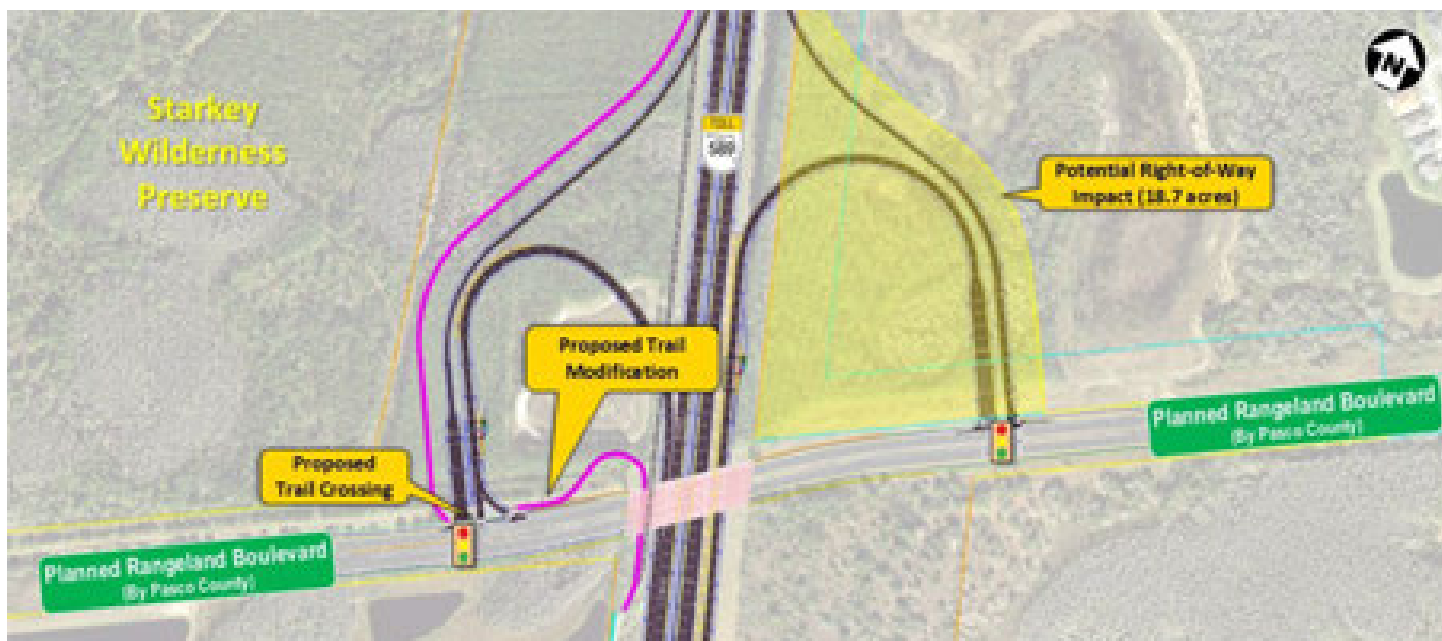
Figure 7. Proposed Interchange Improvements at Rangeland Boulevard
